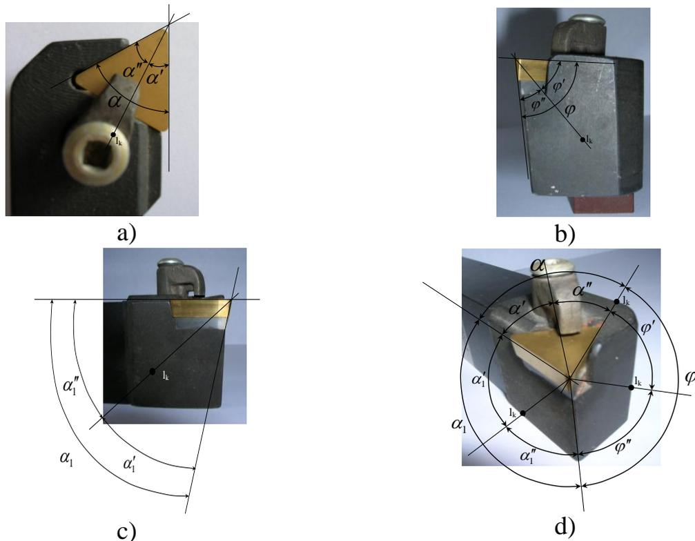
**Fig. 5. Leftside scoring tool with coordinate traces to the location of the converter. a)-top view, b)-type front, c) - side view, d) - form an angle in front and above**
