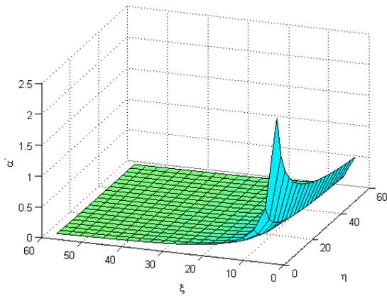
**Fig. 4. Invariance angles to the direction sensor relative to projections of its edges**
