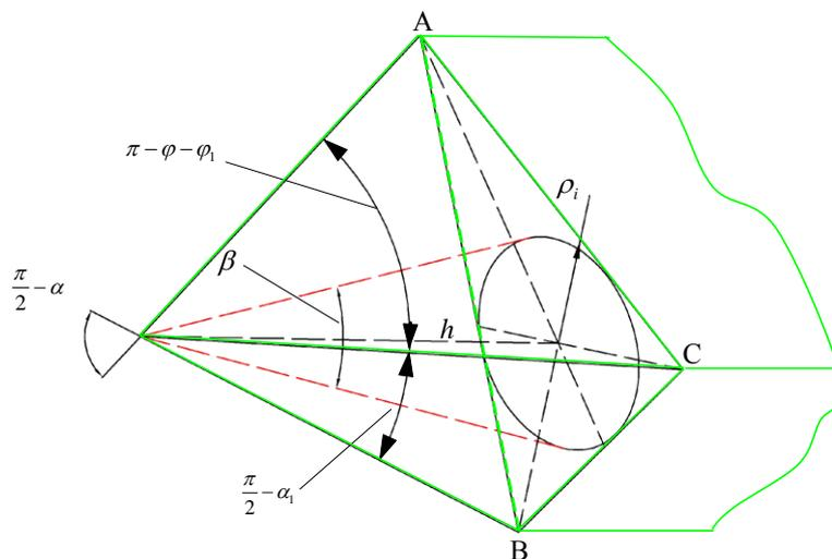
**Fig. 2. Pyramidal model of cutting instrument**
